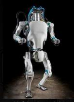
Atlas Robot: a humanoid robot designed to aid emergency services in search and rescue operations
