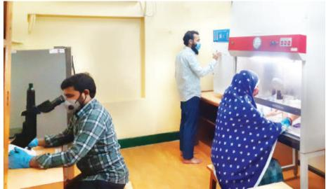
Inverted Microscope: Used for visualizing mammalian cells in culture under sterile conditions and for immunocytochemistry experiments involving mammalian cells.
